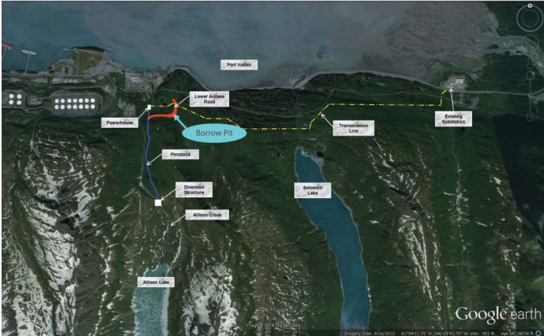
Figure 4. Project area indicating location of gravel material used to fill super sacks - Borrow Pit.
